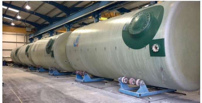
4 x 50m 3 Anaerobic digesters using food and agricultural waste to produce biogas
