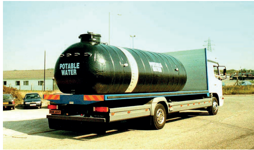
12m 3 potable water tank on flat bed lorry – Dairy, Ulster
