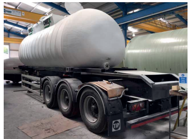
24m 3 low profile 'skeletal' tanker on a steel ISO container frame fitted with 'twist-lock' attachments
