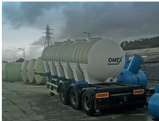
36m 3 conventional cradle mounted tank fitted on an ISO container frame with twist-lock attachments fitted to a skeletal trailer
